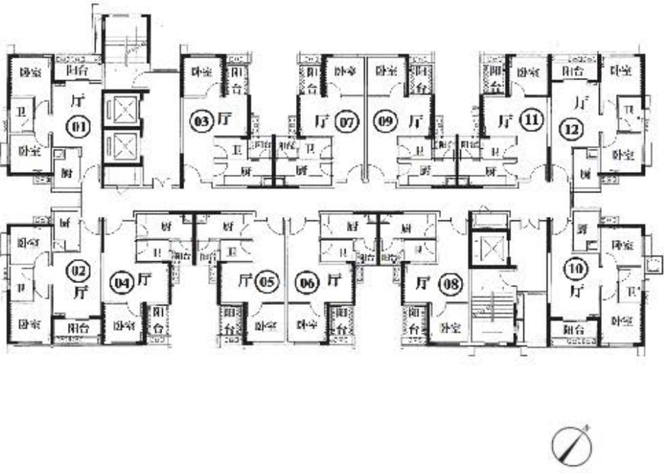
The diagram shows a standard floor plan for Block 18. It features 12 units arranged in two rows. The top row contains units 01, 03, 07, 09, 11, and 12. The bottom row contains units 02, 04, 05, 06, 08, and 10. Each unit is labeled with its number and includes a living area (厅), kitchen (厨), bathroom (卫), and bedroom (房). Units 01 and 12 are two-bedroom units, while all other units are one-bedroom units. The plan also shows common areas, stairs, and a north-south orientation arrow.
